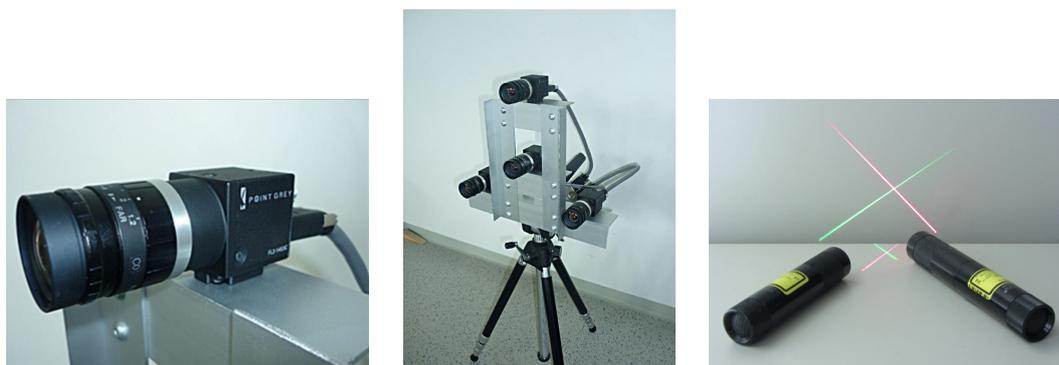
■ **Figure 1** A system of four Point Grey Flea<sup>®</sup>2 FireWire 800 cameras (left) arranged in an upside down Y-constellation (middle). Red and green line-laser probe (right).
